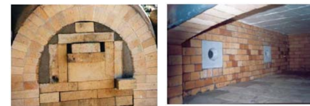
Figure 2a. Refractory lining of a furnace arch (BEE, 2005)
